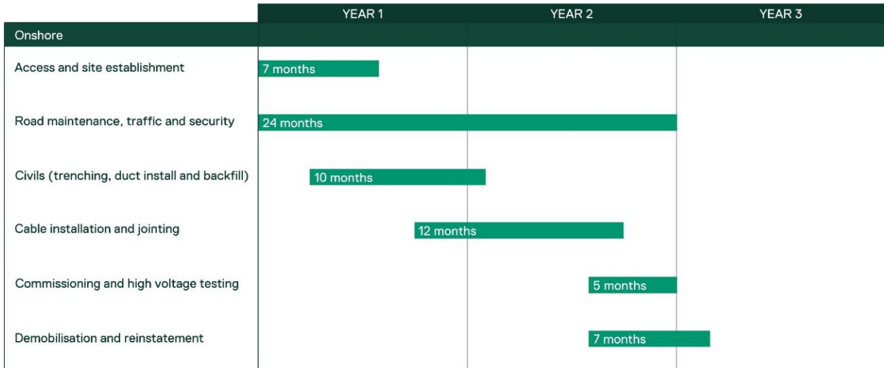
Figure 4-23 Indicative construction schedule – underground cable system
