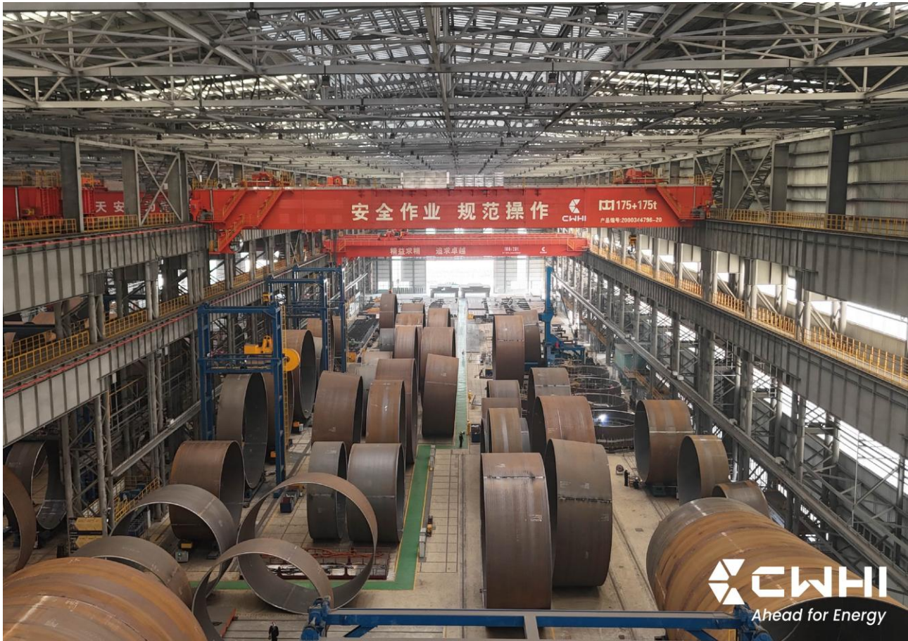
Figure 2-6 A monopile is made up of a series of flat sheets that are rolled and welded forming 'cans'. These cans are then welded together to form a monopile.
