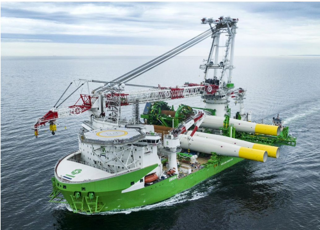
Figure 4-15 Heavy lift dynamic positioning vessel
