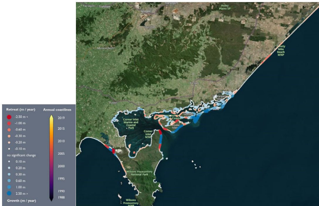
Figure 10: Net shoreline change since 1988 from Corner Inlet to Golden Beach. The barrier islands show significant accretion with minor erosion occurring where the beach-barrier sequence is thin. Source (DEA, 2021)
