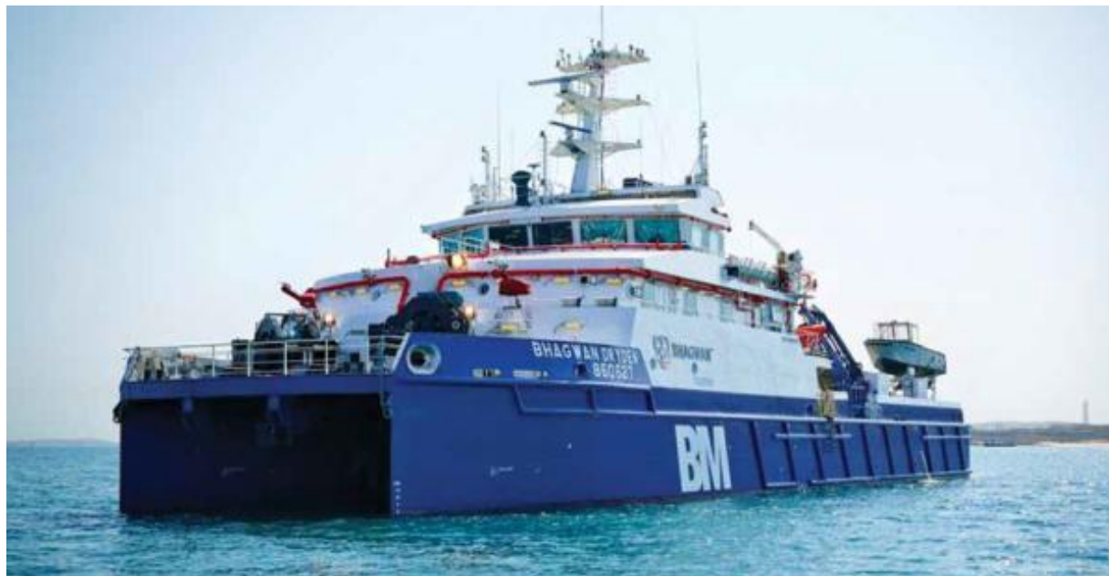
Figure 9-3 Typical cable shore crossing installation vessel
