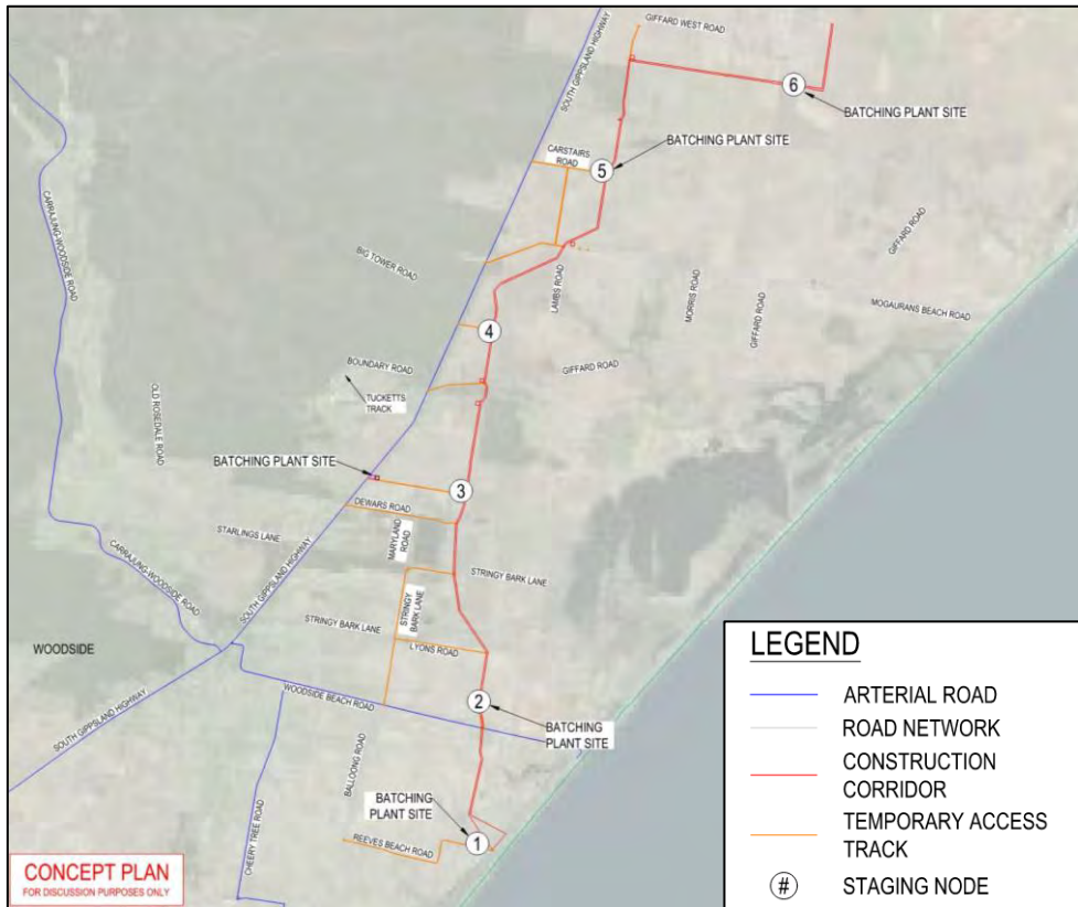
Figure 11 Construction Corridor Staging Nodes
