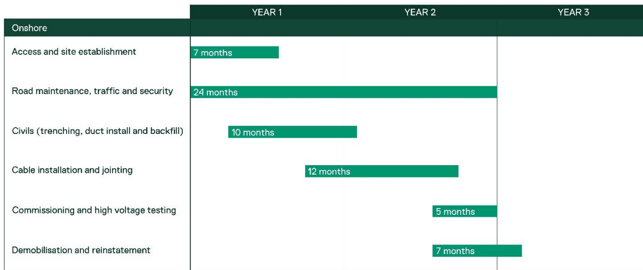
Figure 9-1 Indicated Construction Schedule – Onshore Transmission (source: SOTS, 2025)
